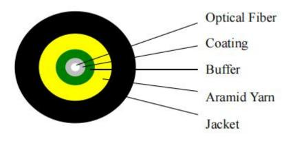
Figure 1 Optical cable section view
